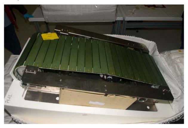
The Combined Operational Load Bearing External Resistance Treadmill (COLBERT) is packed and prepared for stowage aboard Discovery for its transport to the International Space Station.
